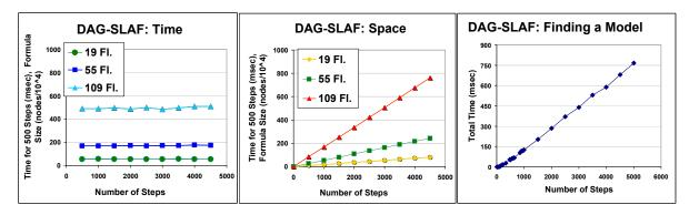
Figure 6: Experimental results for the DAG SLAF algorithm showing time required to process actions, space required to process actions, and time required to extract an action model.
